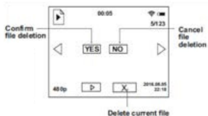
**Note:** During file review some control functions are not available such as menu, zoom control, and IR illuminator control. If the IR was on, it will turn off when entering review mode. The IR illuminator power level is saved and will return to the same power upon exiting review mode.
