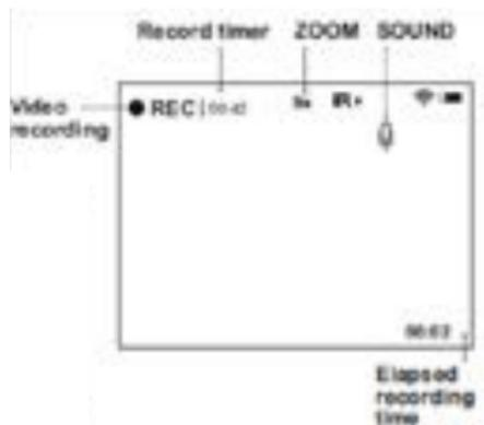
**Note:** the maximum duration of a recorded file is seven minutes. After this time, a video is recorded in a new file. The number of recorded file is limited by the capacity of the unit's internal memory. Approximately 5 hours of video only can be saved on the internal memory.
