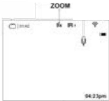
**Note:** digital zoom is not saved in the riflescope's memory. Each time the scope is turned off and back on, digital zoom is turned off and the magnification will be set to the optical magnification (i.e. 4.5x or 6x).
